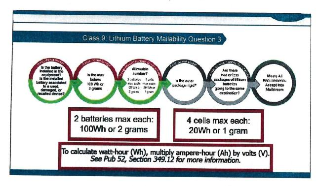
Additionally, multi-cell batteries are limited to 100 watt-hours or two grams of lithium content per battery, while cells or single-cell batteries would be limited to 20 watt-hours or one gram of lithium content each.
